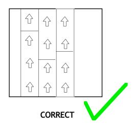
(X) Each roll of Neoflex<sup> $\mathbb{M}$ </sup> is labelled on the underside advising the direction of rolling and which face of the roll is to be placed down on to to sub-floor. Please follow these instructions carefully to avoid potential installation problems.
