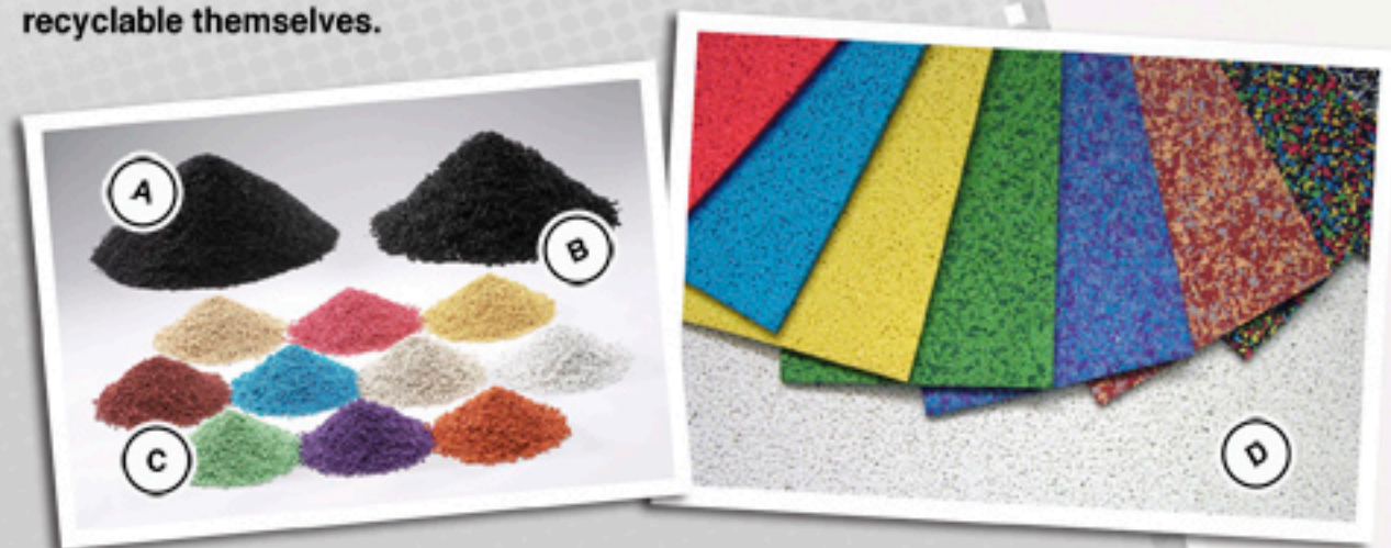
A) Rubber tire buffing B) Rubber chips C) Colored rubber chips D) New products
